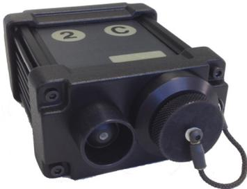
It consists of a control unit and 5 receiver units (paired at the factory), packaged in a foamed carrying case. The housings are extremely rugged aluminium, IP 67 waterproof, dark colors, with dominant black and grey. They are particularly well adapted to harsh environments.
