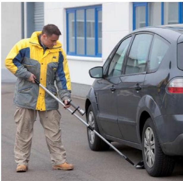
The EFIS® inspection mirrors were designed to support a fast inspection of vehicles and parts of buildings which are difficult to access. There are various fields of application: vehicle undersides, baggage racks, areas over or under furniture, hollows and space in between as well as difficult to access building parts can be inspected rapidly.
