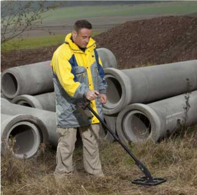
This locator can pinpoint the position of subsurface markers. The great advantage of the system consists in an object-selective location.
