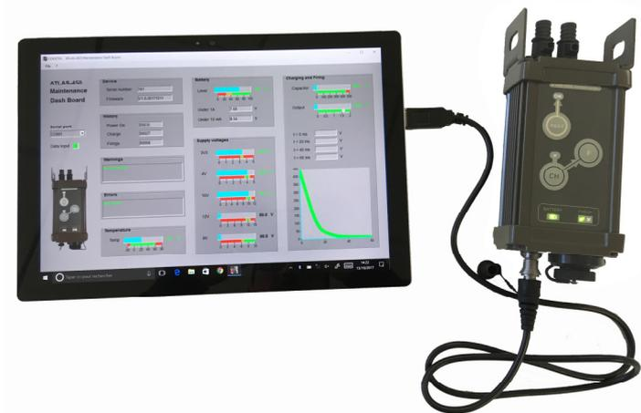
The exploder **ATLAS 450** is power supplied by three CR 123 lithium photo batteries (cheap and widespread). A bicolour led indicates continuously the state of the batteries.
