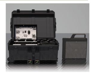
Ideally suited for dismounted operations, the NEOS III is the <u>lightest</u> DR system provided by Logos Imaging. With a built in battery and internal wireless communication, the NEOS III is perfect for users that want to quickly assess an item. At 3.3 kg and only 18 mm thin, the NEOS III can be easily transported on target with minimal effort. The NEOS III produces high resolution 16-bit images and is shielded for up to 330 kV sources.
