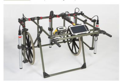
Typically, the MAGNEX/EPAD data recording systems are linked to global positioning systems (GPS) to accurately record the location of detected anomalies. Subsequently, the data are processed to provide an anomaly location map, target anomaly list, and the measured geophysical signal amplitude for each anomaly. These results are then used by UXO specialists to locate, investigate, and remove the metallic anomaly.
