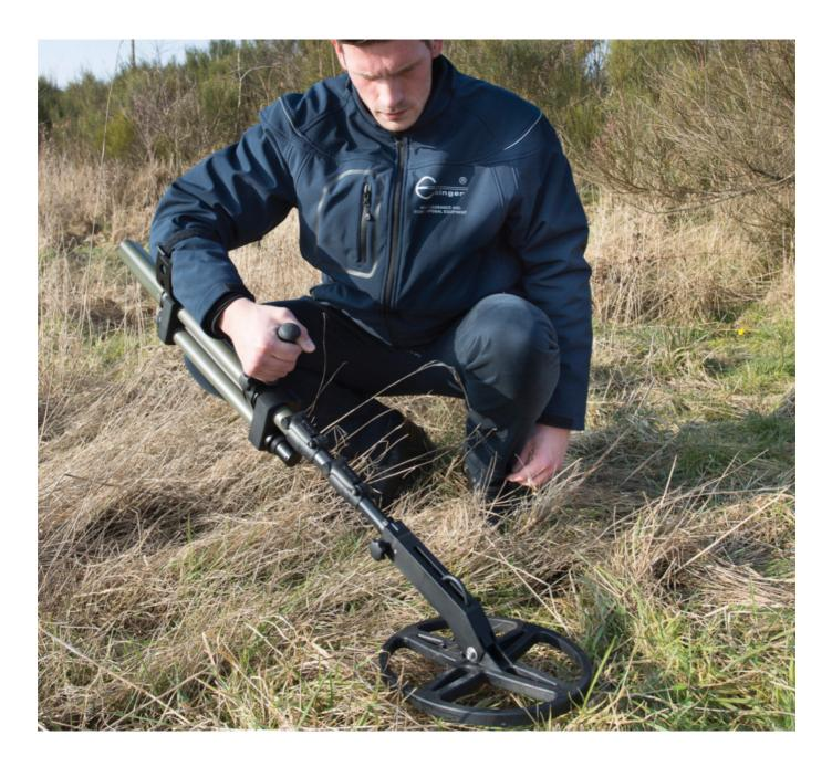
Robust and handy One knob operation Large detection range Static/dynamic search mode Programmable delay steps Non-cooperative soil suppress. Interchangeable search heads Adjustable length
