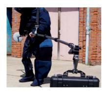
The claw is positioned at the end of a 3 metre telescopic arm. This standoff distance significantly increases operator safety, in the event of an unplanned detonation. The manipulator also hosts a frangible section. In the event of an unplanned detonation, this section will fail first, significantly reducing the transferred along manipulator to the operator.
