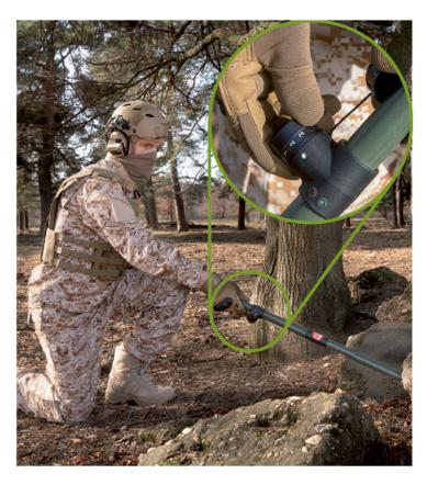
Two dynamic detection steps are foreseen allow for fast subsurface localization of ferromagnetic parts. In this mode continuous magnetic interferences e.g. mineralized soil or fences can be suppressed to certain limits.
