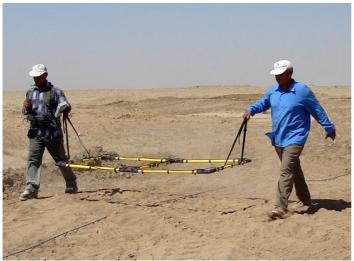
The UPEX 740 M applies the eddy current pulse induction principle. It detects <u>all</u> <u>metals</u>, ferrous and non ferrous.
