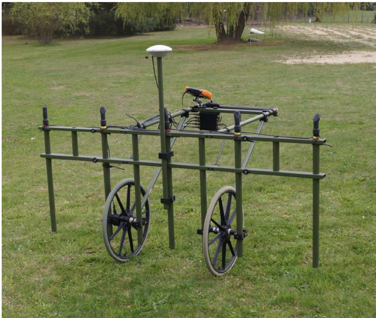
**SYSTEME MULTI-SONDES MXPDA AVEC POSITIONNEMENT GPS**
