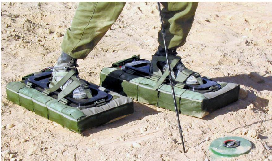
The sandal is made from a reinforced plastic surface. The plastic surface is attached to a canvas and nylon fabric envelope. This flexible envelope contains 5 compartments, each of which contains one air cushion. These cushions are connected to each other via a connecting tube and a flexible manifold. The upper part of the plastic surface is equipped with special straps that harness the shoe to the sandal. In addition, it has a rubber tube with an oral inflation valve and an emergency inflation
