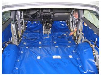
Example of a protection for a Toyota Land Cruiser : the system consists of over 20 different mats, each one sealed by a heavy PVC-cover for protection against wear and moisture.
