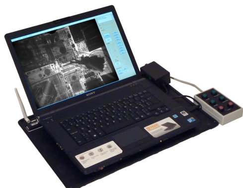
Wireless connection between X-ray generator and image control unit
