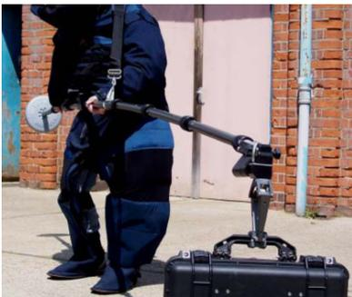
The claw is positioned at the end of a 3 metre telescopic arm. This standoff distance significantly increases operator safety, in the event of an unplanned detonation. The manipulator also hosts a frangible section. In the event of an unplanned detonation, this section will fail first, significantly reducing the force transferred along the manipulator to the operator.
