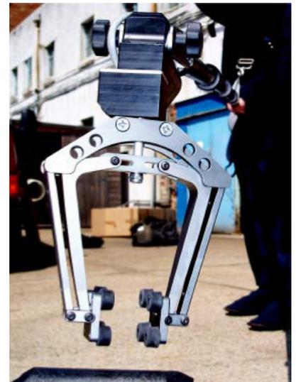
The robotic claw is able to manipulate disrupters, X-ray equipment and a host of other tools used in disposal or investigation techniques. The ability to grasp, and rotate objects in the claw also offers the options of moving devices into containment vessels, or to reposition them in.
