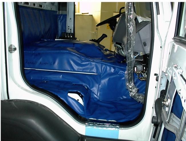
Example of a protection for a Toyota Land Cruiser : the system consists of over 20 different mats, each one sealed by a heavy PVC-cover for protection against wear and moisture.
