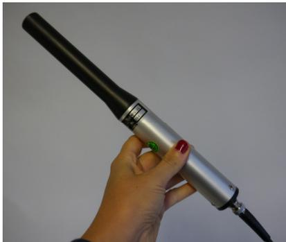
The magnetic sensor is a passive sensor designed for the reception of magnetic pulses coming from timers, and also of signals generated by local receivers' oscillators.
