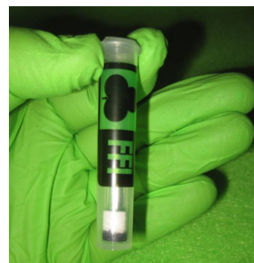
Example of chlorate positive, sampler tip turns from white to dark blue.
